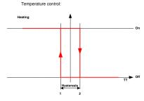
When the temperature is decreasing and reaches point 1 (defined by parameter 43), heating device is turned on and remains active until the temperature in the room is not increased to reach point 2 (defined by parameter 44). In this moment heating device is turned off. When heating device is turned off, then it is working in antifreeze regime. The antifreeze regime turns on heating device when the temperature is lower of equal to the temperature set by parameter 45.
